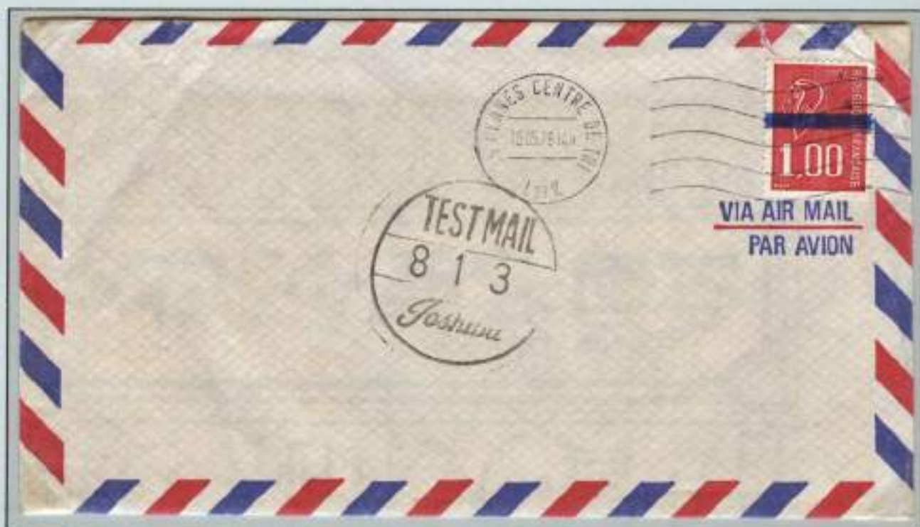
Test mail from the company TOSHIBA, passed in Rennes Centre de Tri for testing purposes. Number 813: 8 stand for country France, 13 represents type of envelope and paper used. For simulating real mail sorting, all kind of sizes, colours, and different paper quality was tested. Stamps are specially pre-cancelled with phosphorescent bar for use in this type of sorting machine. This enables that the letter is always presented in the same disposition. Stamps pre-printed vertical for testing this type of sorting machines.
