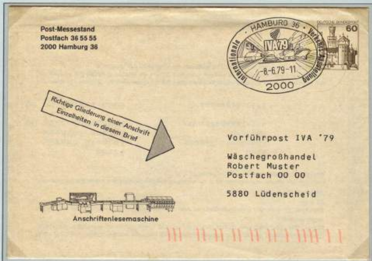
Printed to order (Germany) from Hamburg to Lüdenscheid: code representing 0885 9, left to right code reading. Value 9 points to internal tray or city area. Code gaps represent the value eg: lllxx = 4+7 = 0 ; lxllx = 7+1 = 8
