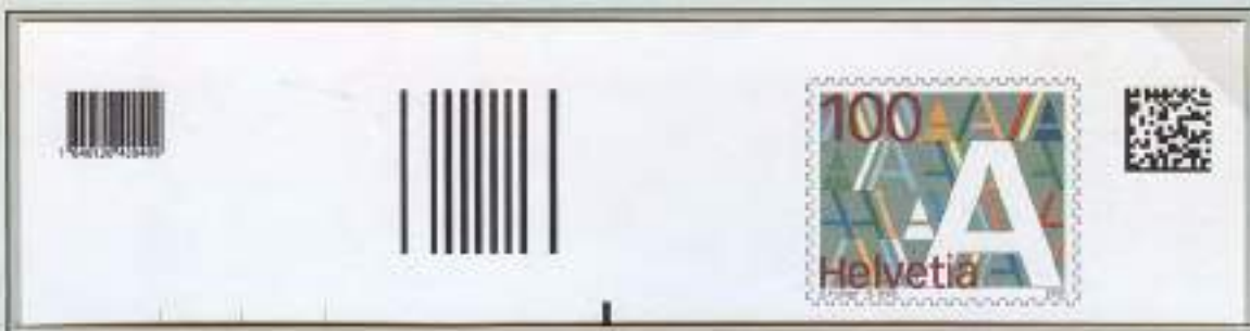
Stationery (Switzerland) with 3 types of bars; EAN-13 (left), 2-Dimensional CP-code (right) and sorting bar code (center)
