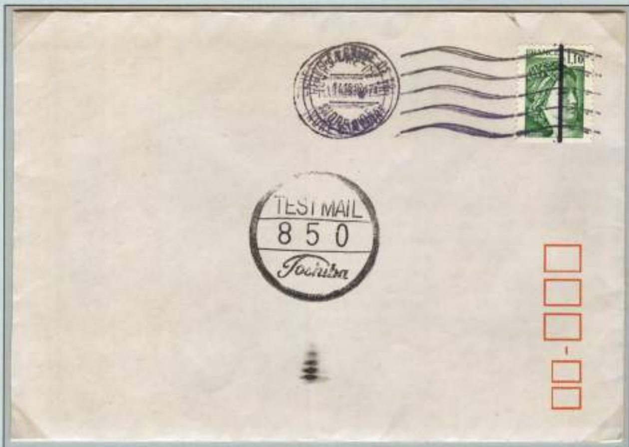
Test letter used in the CFC (culler-facer-canceller) installed in Tours Centre de Tri in the period October 1982. Fuzzy cancellation caused by multiple use of the training post. Cancel of first generation with Toshiba logo. Number 850: 8 stand for country France, 50 represents type of envelope and paper used. Stamps pre-printed vertical for testing this type of sorting machines.
