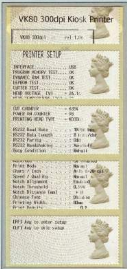
Print out on 1st Class stamps (Great-Britain) of printer test of a self-service payment NCR VK80 thermal printer widely installed in post offices.
