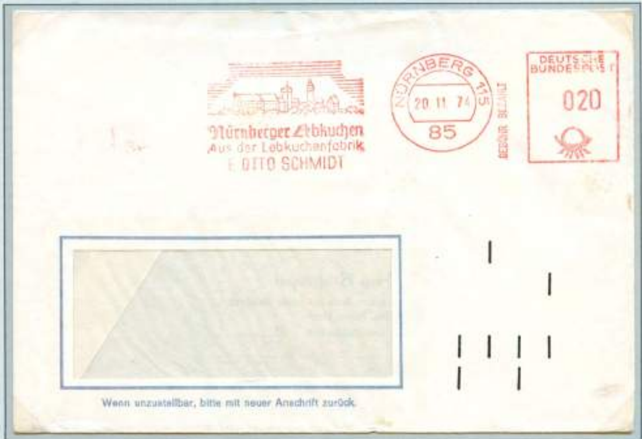
Letter send from Nürnberg: code representing 0405 or 5040, which point to internal tray of the sorting machine.
